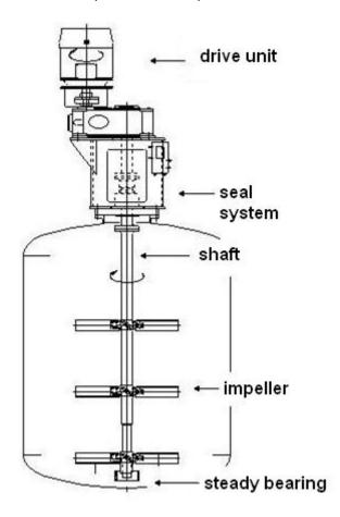
**Control unit:** this consists of a motor to provide energy, which may be electric, pneumatic or hydraulic, and possibly a reduction gear to achieve the required speed.
