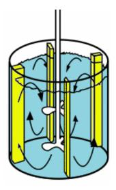
The aim of the axial impeller is to push the fluid towards the bottom, from where it then rises back up along the walls When the movement along the walls reaches the free surface, it heads back down along the shaft axis.
